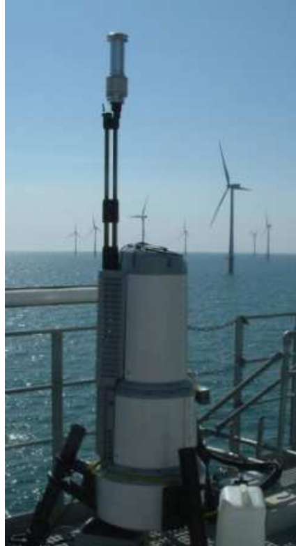
A ZephIR lidar installed at the UK's Robin Rigg offshore wind farm (Sources: ZephIR, Natural Power)
