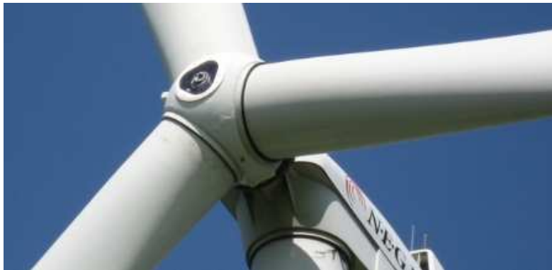
The hub of the NM 80 wind turbine, with the optical head of QinetiQ's (Natural Power) ZephIR lidar in the tip of the wind turbine (Source: Risø)
